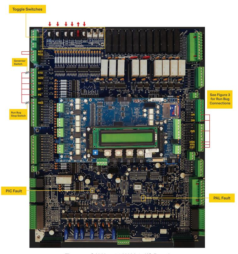
Figure 4: GALX-1102AN Main I/O Board
